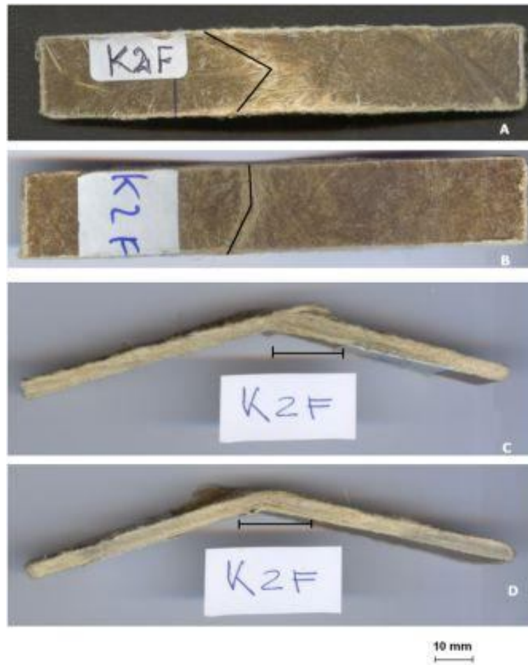
Figure 3: Fractured surfaces of flexural samples of hemp/epoxy laminate (showing delamination in two directions, highlighted in (a) and (b); the extent of delamination is highlighted in (c) and (d).
