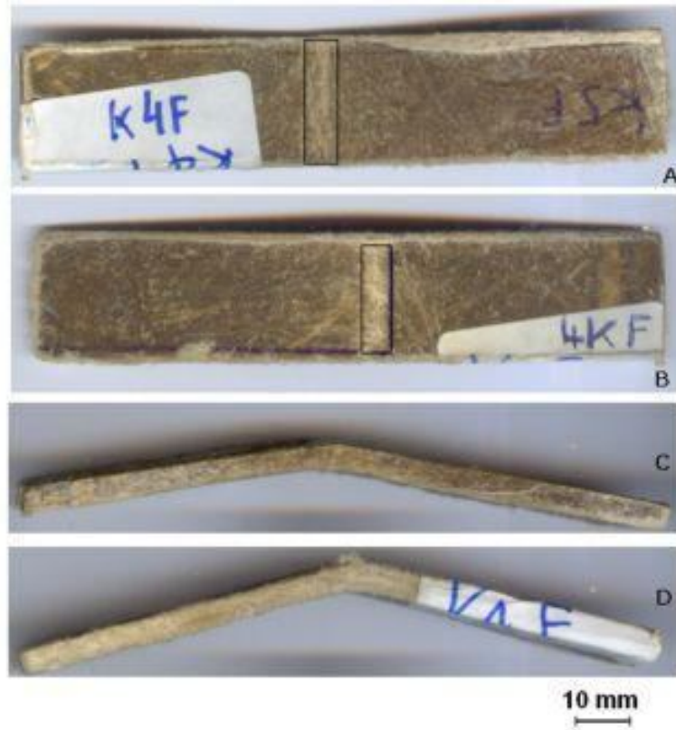
Figure 4: Fractured surfaces of flexural sample of hemp/epoxy laminate (showing wider delamination area, reported as the black edges rectangle in figure)
