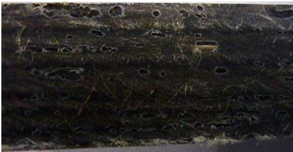
Figure 8 Superficial voids, indicating insufficient fibre impregnation on flax-epoxy composite (2.3 mm. thread)
