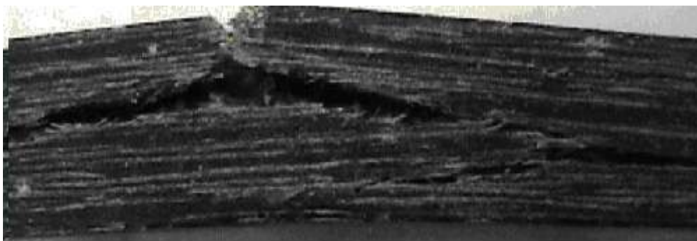
Figure 9 Extensive impact cracking due to fibre tearing off on flax-epoxy composites (0.2 mm. thread)
