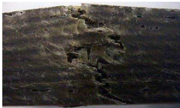
Fig. 2 Impact damage, triggered by sub-surface defects, on the surface of a flax-epoxy laminate
