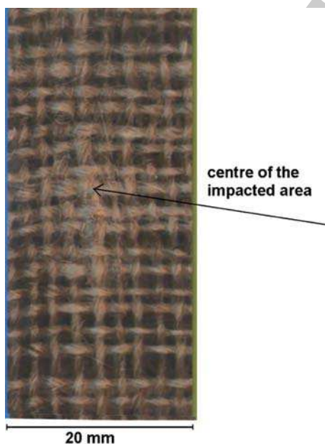
Fig. 1 Slight appearance of impact damage (energy = 10 J) on the surface of a jute/polyester laminate
