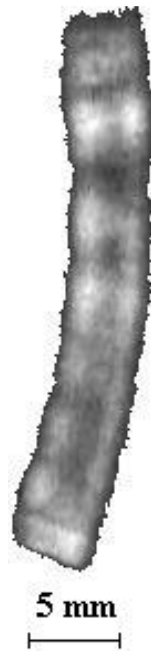
Figure 9. Micrograph of a partially deswollen 7:1 gel (1% crosslinker) at approximately 5:1 dilution
